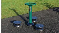
Rubber bound mulch, or just simply mulch as it is referred to in our industry, has a very natural appearance resembling the shape of rough cut bark chippings that were once widely used as playground surfacing. In reality, the shape is the only part of mulch that resembles bark chips.
