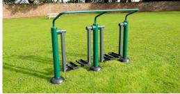
Can we class grass as a safety surface or just a surface? You may say just a surface but it is considered a safety surface for critical fall height of up to 1.5m with a set criteria as it can be impact absorbing (https://www.rospa.com/play-safety/advice/grass).
